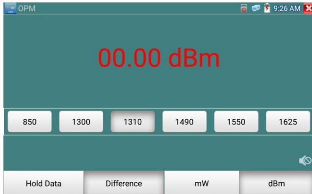
Data hold and Relative measuring use together, the data is yellow while the function is effect.
