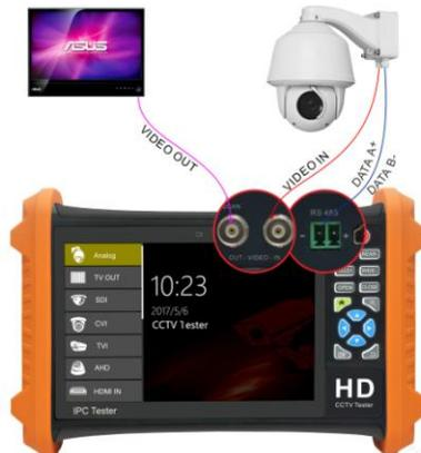
(2) Connect the SDI camera or the speed dome RS485 controller cable to the tester RS485 interface.
