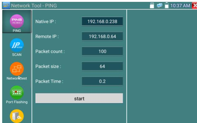
**Application:** PING testing is the most conventional network debugging tools. It is used for testing if the connected IP camera or other network equipment's Ethernet port is working normally and the IP address is correct.
