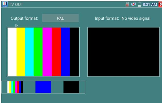
Move the cursor to the bottom of the color bar, blue, black to choose the appropriate image output; Press the Back button to close and return to the main menu.
