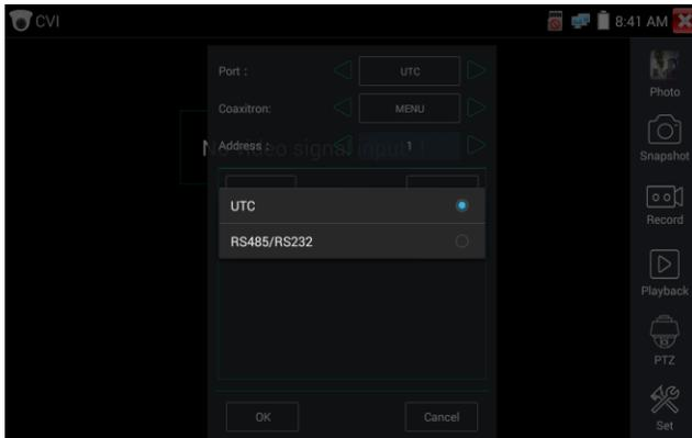
Press the arrow keys to move the cursor to set the PTZ address parameter
