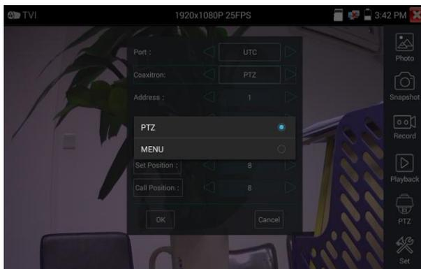
Enter the address code of the menu, after set the parameter, move the cursor to the icon
