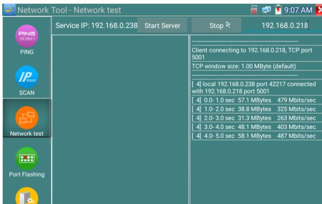
Network bandwidth testing can also be tested with a computer using compatible network bandwidth testing software. Install network bandwidth testing software on a computer, as a test Client or Server, to do the mutual testing with the tester. If use computer as the server, the computer IP address
