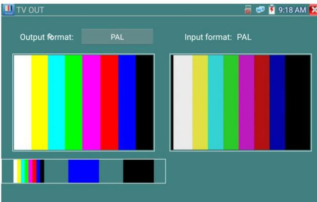
**BNC loop test:** Tester can send and receive color bar generator through the tester’s “video out and video in” port, it is for testing transmission channels, such as video Optical, video cables etc. The tester “VIDEO OUT” port to connect optical terminal’s sending port, and “VIDEO IN” Port to optical terminal’ s connect its receiving port.
