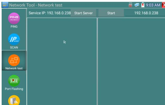
When test, need a tester or a computer installed Network Test Software as the Server, the other tester sends packet test. The two testers must be in the same network segment.
