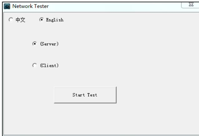
Tester as Client, tester's IP address is:192.168.0.238. The Server and the Client are at the same network segment, but with different IP address. Input Server's IP address 192.168.0.218 in the tester and click “Start” to test network bandwidth.
