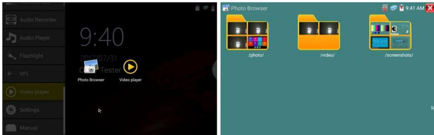
The Media player can browse video and image files. It supports the video formats of MP4, H.264, MPEG4, and MKV. The cctv tester recorded files can play directly via the Media player. The Media player will automatically display the video files from the SD card. Press the Menu key to select the file to be played, which is played on the screen. Press the Back key to quit.
