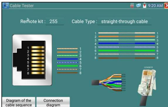
Test LAN cable or telephone cable.
