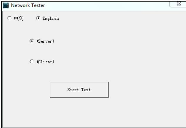
Tester as Client, tester's IP address is:192.168.0.238. The Server and the Client are at the same network segment, but with different IP address. Input Server's IP address 192.168.0.218 in the tester and click "Start" to test network bandwidth.
