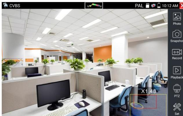
press the key to zoom out , press the key to zoom in, press upward and downward key to move the image
