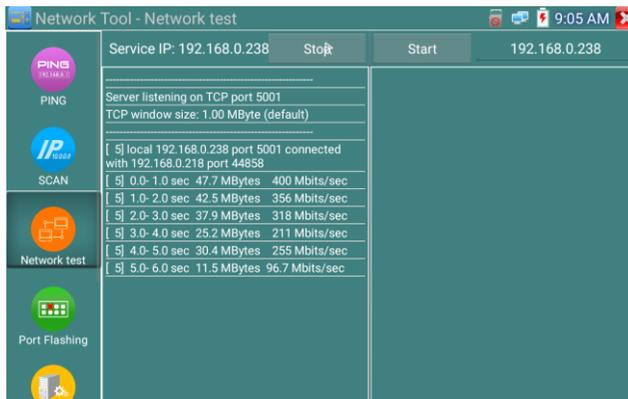
**b). Start send packet test:** Using the other tester, type in the Server's IP address at the top right corner of the screen. This app is used to send packets for network speed testing. Click the “Start” button to send the packets and start testing.
