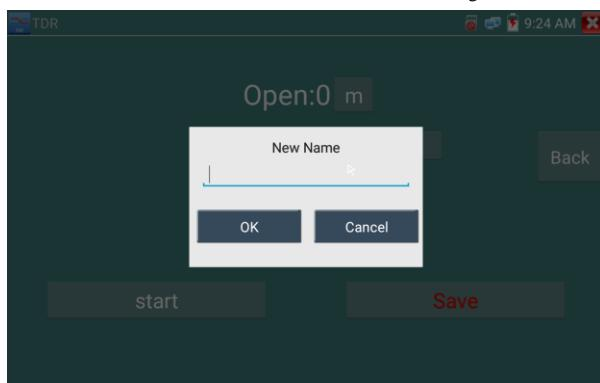
**Application:**TDR test is the use of pulse reflection method, to transmit pulse signal for tested cable, when cable is open circuit or short-circuit, reflected pulse is generated, the tester receives and deals with the reflected wave, measurement results displayed on the screen. TDR can test cable open circuit and short circuit, help engineer quickly find the cable's problem location. It is more convenient and efficient to repair the faulty cable.
