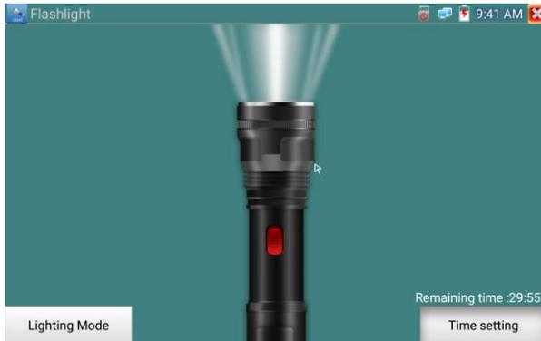
While in the flashlight app, click the red button to turn on the LED lamp. Press it again to turn it off. Press the Back button to exit the application, the lamp will stay on. Click the Time Setting button to set a timer that will shut off the lamp.
