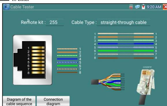
Test LAN cable or telephone cable.
