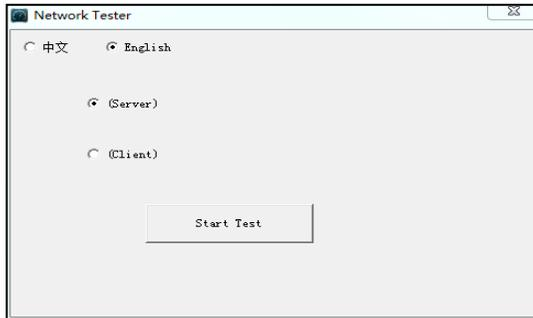
Tester as Client, tester's IP address is: 192.168.0.238. The Server and the Client are at the same network segment, but with different IP address. Input Server's IP address 192.168.0.39 in the tester and click "Start" to test network bandwidth.
