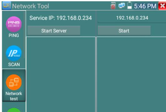
**a).Start the server:** Click “Start Server” button to use the tester as a Server. It will display its IP address at the top of the screen.
