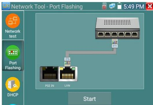
If the tester and PoE switch are connected well, the LAN port of POE switch flash at special frequency,
