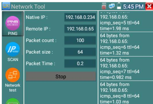
**Application:** PING testing is the most conventional network debugging tools. It is used for testing if the connected IP camera or other network equipment’s Ethernet port is working normally and the IP address is correct.
