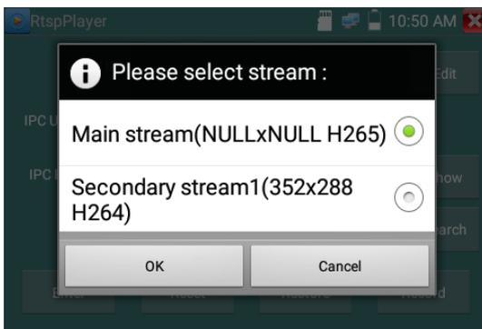
**Note: In the event the ip tester does not auto detect the rtsp stream, refer to the specific camera manufacturer for the specific rtsp stream url. you may find this on line with a search of the camera model number and the word rtsp.**
