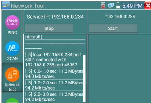
**b). Start send packet test:** Using the other IP tester, type in the Server's IP address at the top right corner of the screen. This app is used to send packets for network speed testing. Click the “Start” button to send the packets and start testing.
