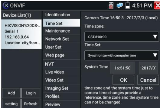
**Maintenance:** For camera software reset or restore to factory settings.
