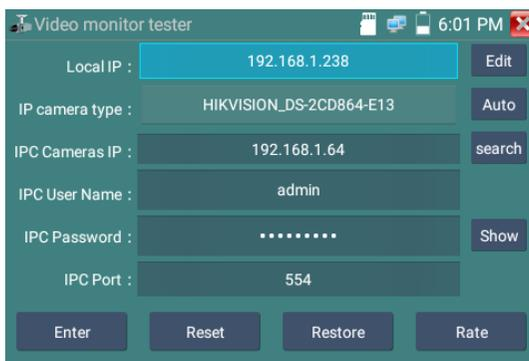
**Local IP:** This is the tester's IP address. Click "Edit" to enter "IP setting" and change the tester's IP address settings
