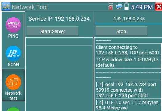
Network bandwidth testing can also be tested with a computer using compatible network bandwidth testing software. Install network bandwidth testing software on a computer, as a test Client or Server, to do the mutual testing with the tester. If use computer as the server, the computer IP address is :
