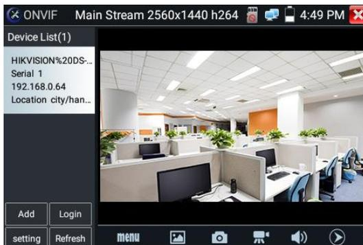
If you select ONVIF Rapid mode, the meter automatically scan different network segments for ONVIF cameras. It lists the camera name and IP address on the Device List. Tester can auto login camera and display camera image.
