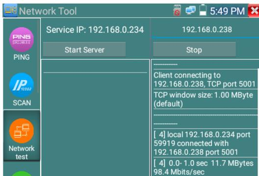
Or use tester as a Server, computer as test Client (select Client, input tester's IP address to test)
