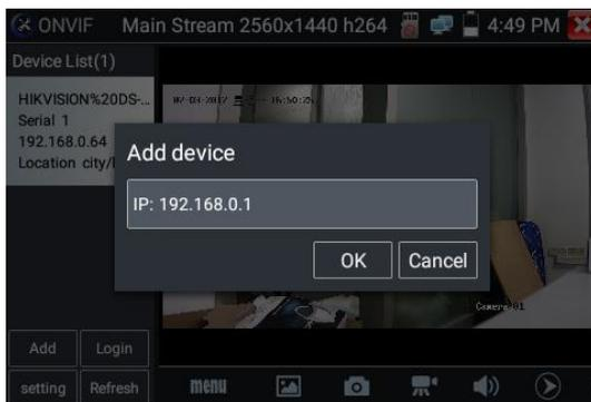
Click the button “Refresh”, tester will scan the ONVIF camera again. Click the newly displayed ONVIF camera on the “Device List”. The tester will show the IP camera’s relative information and settings.
