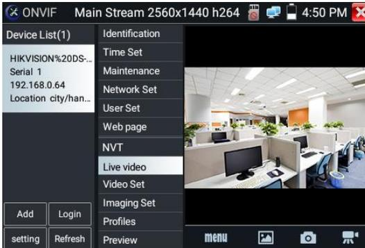
**ONVIF PTZ control:** Tap the image in the direction you want the PTZ camera to move. Tap the left side of the image to move left, right to go right, up to go up and down to go down. Compatible IP PTZ cameras will rotate accordingly. PTZ rotation direction is displayed on top left corner of the image.
