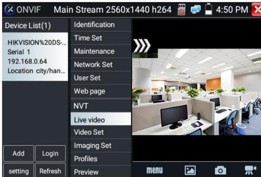
**IP camera video settings:** Click “Video Set” to enter the IP camera’s encoder and resolution settings. Make the desired changes and click “OK” to save.
