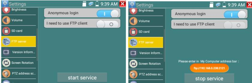
Start the FTP server and then input the tester’s FTP address in the PC’s address bar. This will enable the PC to read, copy and edit the files from the SD card without the use of SD card reader.
