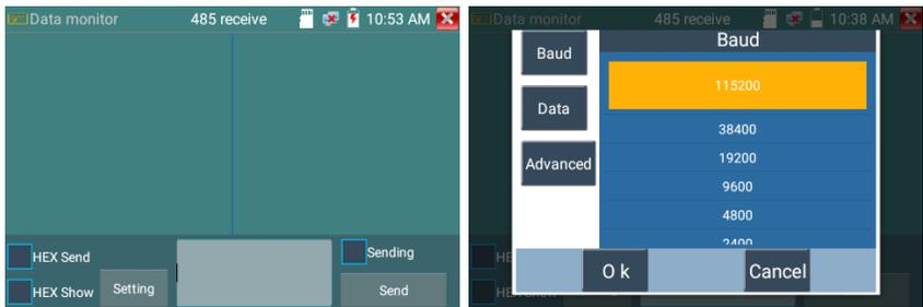
Click “Setting” to choose the baud rate of RS485; it must be the same as the DVR or the Control keyboard. The DVR or Control keyboard send the code to the tester, if it can be read, the protocol will shown on the upper right, like Pelco D, if not, like P:---
