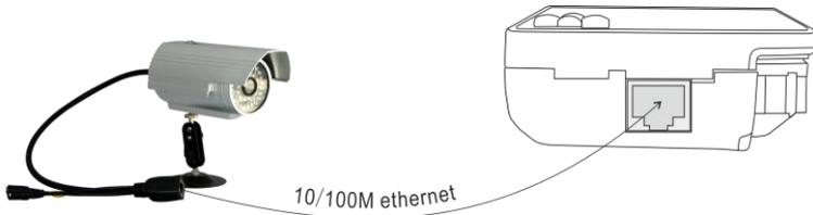
**Note:**1) If the IP camera requires PoE power, then connect the IP camera to the IP tester's LAN port . The tester will supply PoE Power for the IP camera. Click on the icon labeled POE to turn the PoE Power off or on.
