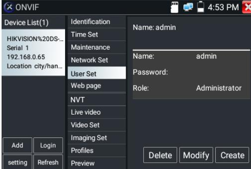
**Network setting:** Click “Network Set” to change the IP address. Some cameras cannot support change IP address, so there is no change after saving.
