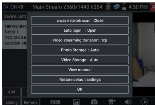
**Across network segments scan:** After open this function, enter “Setting”-“IP Settings”-“Advanced” to add other network segments IP, Rapid ONVIF function can across network segments to scan camera’s IP.
