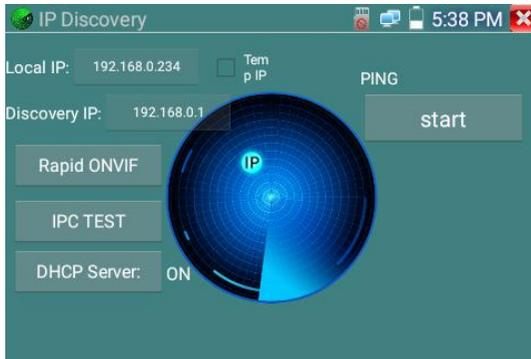
**Local IP:** Tester's IP address, Tester can auto-modify the tester's IP to the same network segment with the scanned camera's IP
