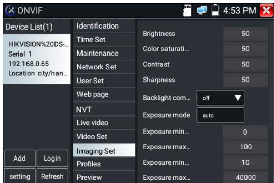
**Profiles:** Click "profiles", can view video streaming current configuration files, as well as switch between Major stream and minor stream .
