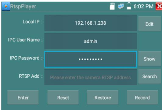
**Local IP:** This is the IP testers IP address.
